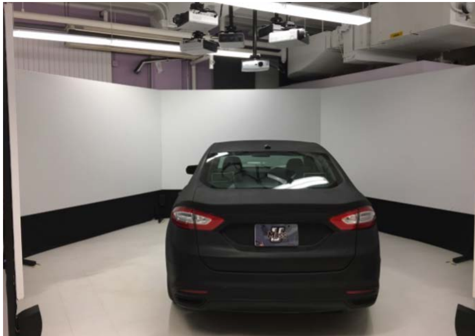
Figure 3.1 – Full-immersion driving simulator
